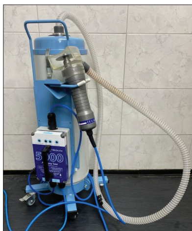
Figure 2. Oscillator saw with suction of the bone aerosol
